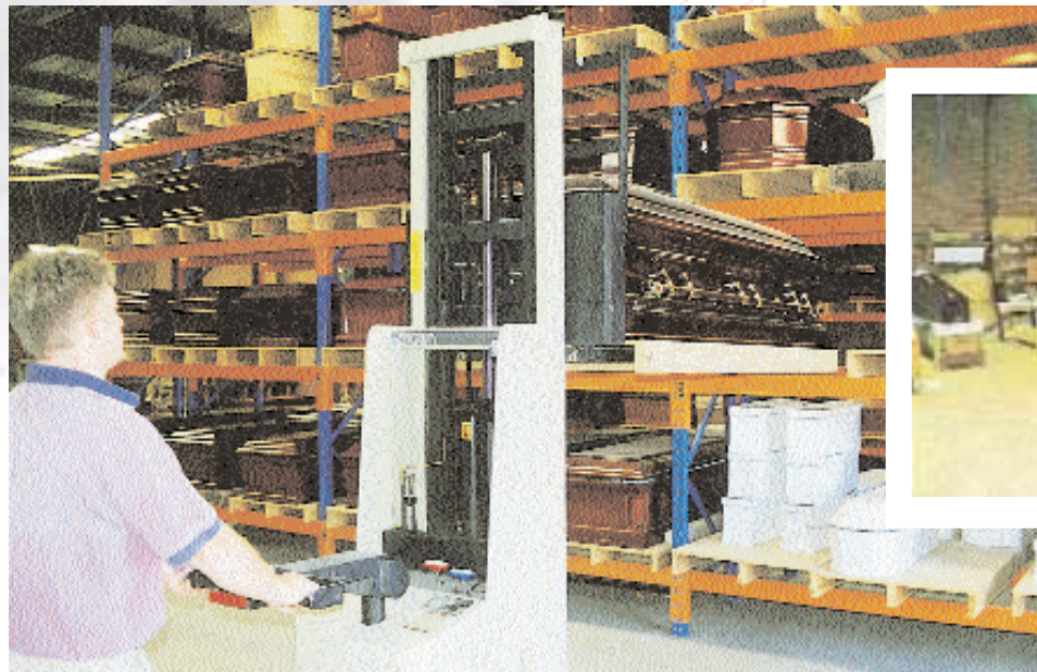
Left The forks have been fitted with slippers to assist the handling of 2m long pallets.
