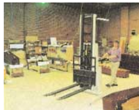
Left The forks have been fitted with slippers to assist the handling of 2m long pallets.
