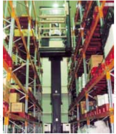
Left & below The very narrow aisle Turret Truck maximises storage capacity within Miascor's temperature and humidity-controlled warehouse
