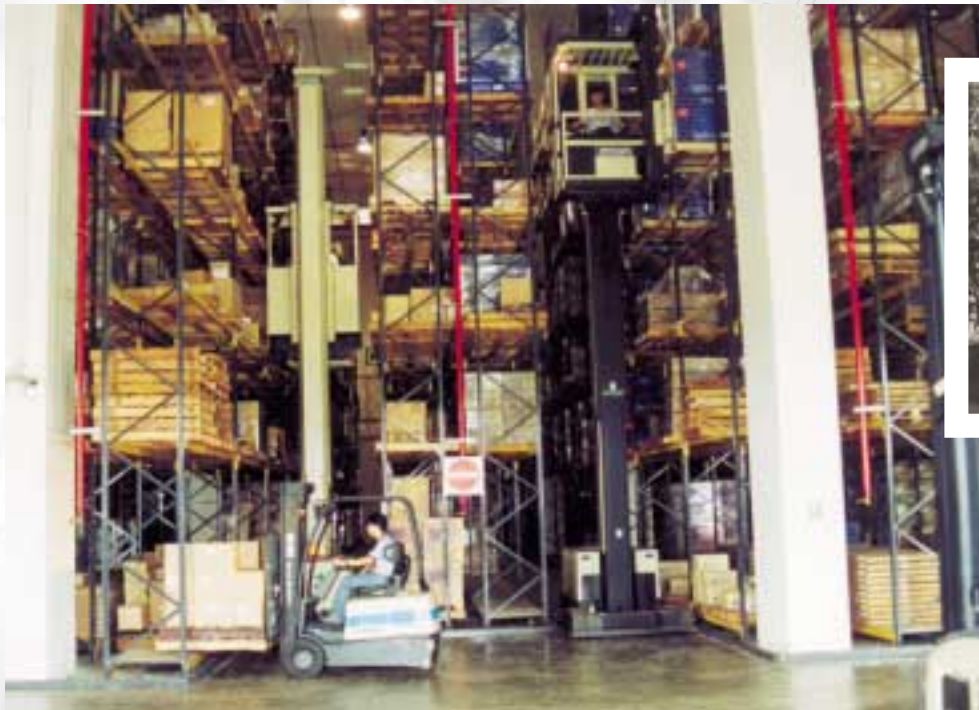
Left Four TSP Turret Trucks are used for pallet handling and case picking in BAX Global's 15m high warehouse.
