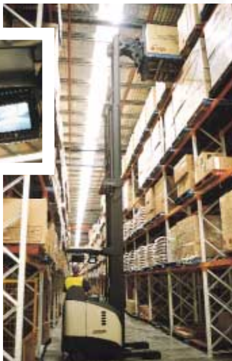
Above & right The use of on-board cameras and height selectors has helped to improve productivity and safety.
