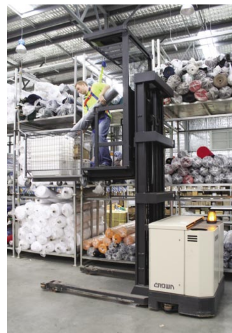
Perm-A-Pleat storeman utilising one of the tailored Crown stockpickers to pick roles of fabric from steel cages.
