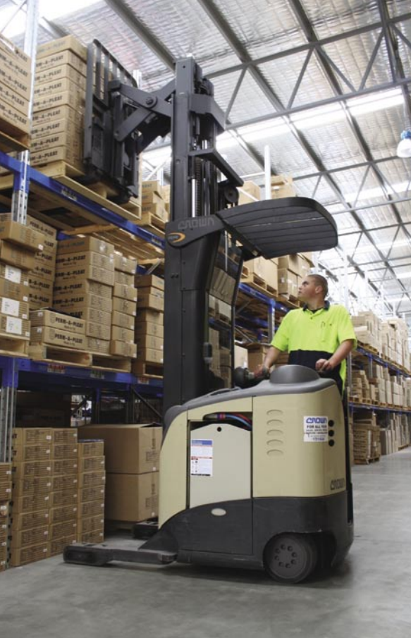
Crown Ride on Reach truck demonstrating its narrow aisle working ability.
