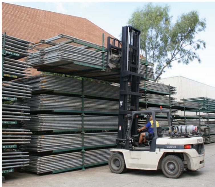
The Crown 7 ton LPG truck is fitted with hydraulically adjustable forks to handle the long and wide loads that are required in the scaffolding industry.
