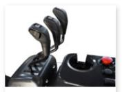
Hydraulic controls Manual levers are the standard hydraulic controls for the C-B series. Fingertip controls are also available as an option.
