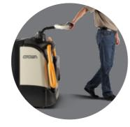
Manoeuvrability advantages result from the fold-up rider platform, contoured power unit and ergonomic tiller positioning providing ample foot clearance.
