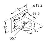
Mounting plate allows all types of couplers to be adjusted in 45 mm increments (Rockinger RO 244 in 55 mm increments)
