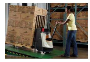
Crown's ramp hold improves operator confidence and control by reducing the possibility of unexpected reverse travel when stopped on an incline. It also allows consistent speed on ramps, with or without a load.
