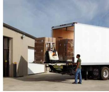
Thousands of applications without receiving/shipping docks require delivery from truck to curbside via lift gates. Crown's compact design and maneuverability featuring position speed control and vertical tiller drive make the WP 3200 Series ideal for these applications.
