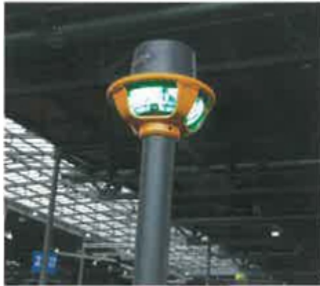
The green lamp lights up to indicate that the truck is ready for remote-controlled operation
