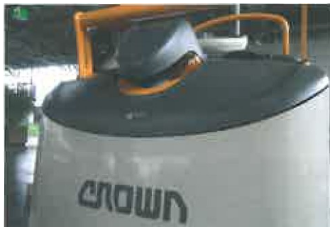
The scanner keeps a watchful eye on things, ensuring the truck stops automatically when it spots an obstacle
