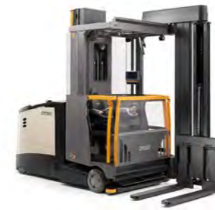
TSP 1000 Series VNA Truck Max. truck capacity: 1,500 kg Max. lift height: 13,485 mm
