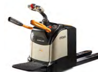
WT 3000 Series Pallet truck with folding platform Max. truck capacity: 2,500 kg
