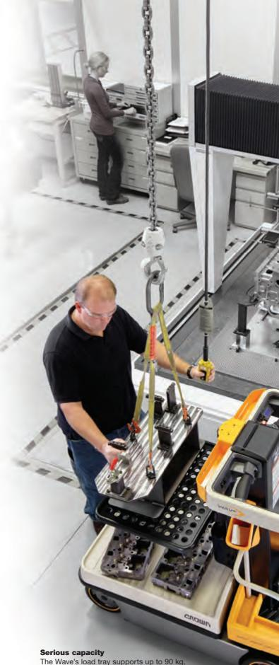
The Wave's load tray supports up to 90 kg, while the load deck holds up to 115 kg, going far beyond what workers can safely lift and move using ladders.
