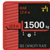
**Red** – load exceeds capacity or is above lift height limit.
