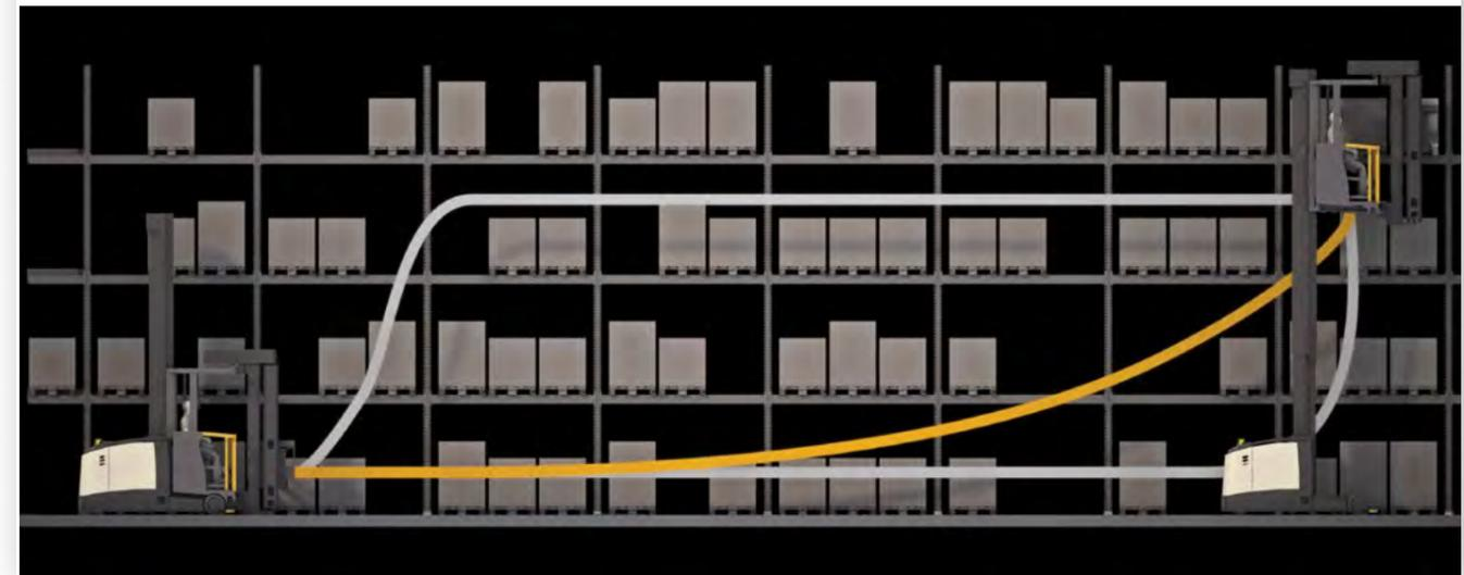
**Auto Fence** helps promote safety by slowing or stopping travel and limiting lift height within a very narrow aisle based on the lift truck's location.
