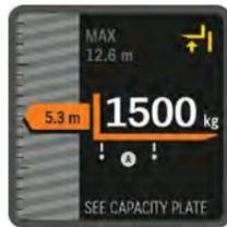
**Grey** – load is below capacity and lift height limit.
