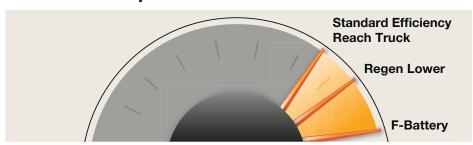
The Crown RM 6000 reach truck's standard regenerative lowering and F-battery compartment gives you improved energy efficiency for increased runtime and reduced costs.
