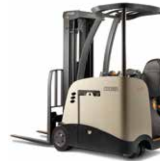
RC 5500 Series 3-Wheel Stand-Up Counterbalanced Truck Load Capacity: 3000 to 4000 lb Lift Height: 154 to 276 in
