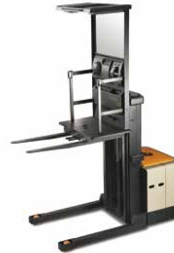
SP 3570F Series Straddle Voltage: 24 volts Load Capacity: 3000 lb Lift Height: 210 to 366 in
