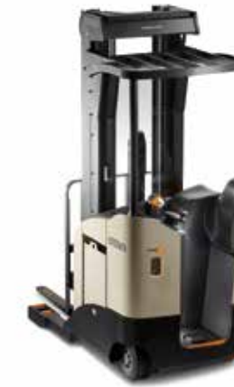
RR 5725 Series Reach Truck Load Capacity: 3500 and 4500 lb Lift Height: 198 to 400 in
