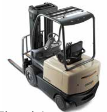
FC 4500 Series 4-Wheel Sit-Down Counterbalanced Truck Load Capacity: 4000 to 6000 lb Lift Height: 118 to 312 in
