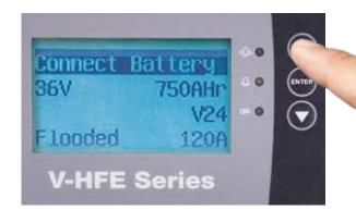
Chargers are configured from the front panel screen and keypad. No cables, software or complex internal switch configurations are required.
