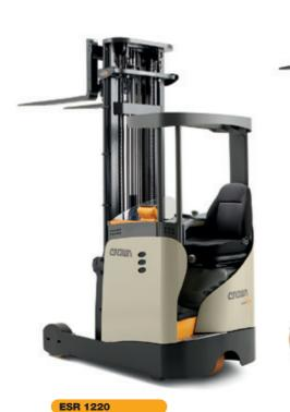
Available in 1.4 tonne and 1.6 tonne capacity,
