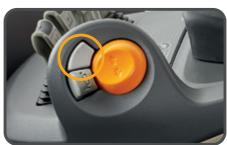
Optional Auto Height Select enables the forks to stop automatically at programmed rack heights using the one-touch button or on-screen selections. Precise, automated positioning helps prevent damage to products, racking and forklifts while simultaneously increasing throughput.
