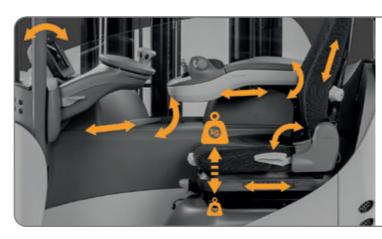
The right fit, personalised for both small and large operators - operators benefit from optimised control with adjustable settings for the seat, controls, armrest and display screen.
