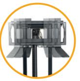
5th Hydraulic Function option to control attachments such as fork positioners with sideshift or clamps to meet specific application requirements
