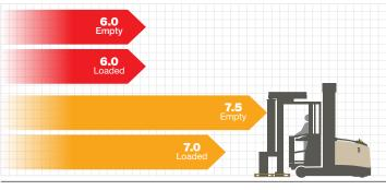
**Maximum Travel Speed (mph)** Faster travel speed means trucks get to the pick slot quicker for a 25 percent advantage.
