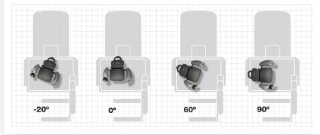
**Innovative Steering Tiller** another Crown exclusive, can be operated with the finger divot or via a flip-up tiller knob.
