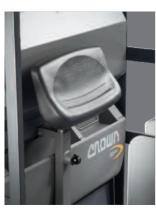
**Backrest** for Load-Facing **Operator Controls**
