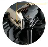
An optional torsion bar with quick-adjust casters (shown) adds rigidity. Each caster can easily be adjusted to compensate for normal drive tyre wear.
