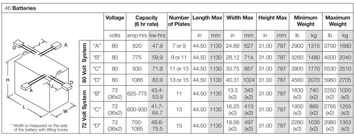
Connector Location / Length (J): A/15" (A/381mm) for all battery sizes except 80 Volt "D" Batteries require D/22" (D/559 mm). Standard Connectors: All 80 Volt Batteries = SB350 Black, All 72 Volt Batteries = SB350 Gray.
