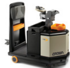
TR 4500 Series Tow Tractor Rolling Load Capacity: 10,000 lb
