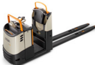
GPC 3000 Series Low Level Order Picker Load Capacity: 6,000 lb Platform Lift Available
