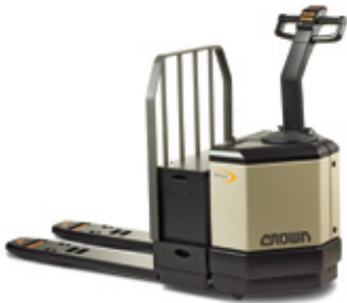
PW 3500 Series Walkie Pallet Truck Load Capacity: 6,000 to 8,000 lb
