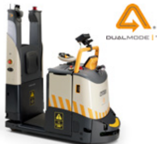
DualMode T 1000 Series Tow Tractor Rolling Load Capacity: 11,000 lb
