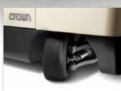
**Rugged Steering Axle** Large steering spindles equipped with king pin and sealed taper roller bearing design absorb impacts and keep moving parts free of contamination. A thick steel weldment axle beam offers strength and durability.
