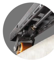
One-piece high tensile steel forks are formed into a C-channel and reinforced in critical areas. An adjustable pull-rod lift linkage eliminates buckling forces and elevates the riser axle for protection.
