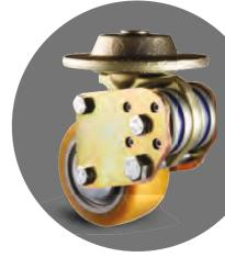
Shock-absorbing casters with lifetime torsion springs reduce impacts to the chassis and extend caster life.
