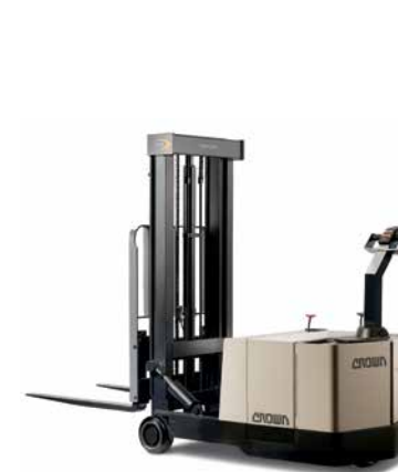
WB Series Intermediate-Duty Walkie Stacker Load Capacity: 900, 1300 & 1800 kg Lift Height: 2692 to 4521 mm
