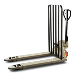
Load Backrest is constructed of 8mm steel, and backrests are available in 1220 mm and 1525 mm sizes. Bolt-on installation simplifies field retrofits.
