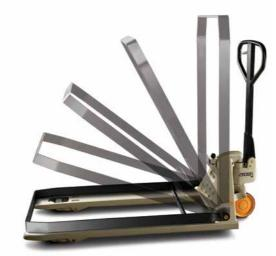
Skid Adapter increases lowered height to 140 mm to permit skid handling. Raised height increases to 267 mm. Adapter latches in vertical position for pallet-handling tasks.
