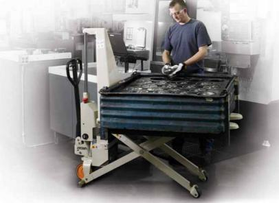
Scissor Lift improves operator comfort and efficiency by avoiding unnecessary bending and lifting that can cause strains and stresses on the body. It has various uses as a hand pallet truck and a mobile work positioner, can handle skids and open-bottom containers, and can be used to hold materials that will be fed onto conveyors and printing or punch presses.
