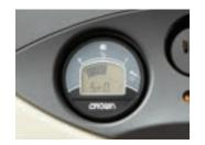
The standard display features fault code readout to clearly identify a system fault during truck operation or start up. No more guesswork, the display says it all.
