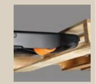
The smooth, rounded fork tips simplify pallet entry and are boxed in to add strength. In addition, the design of the fork tips prevents build up of debris.
