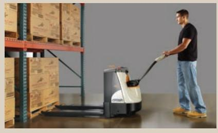
**Pallet entry** is enhanced by increased visibility of the fork tips resulting from the combination of a low profile power unit and Crown's exclusive fork tip indicators.
