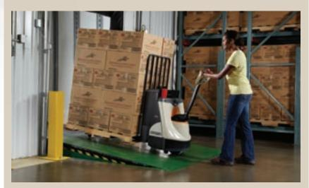
**Crown's ramp hold improves operator confidence and control** by minimizing the possibility of unexpected reverse travel when stopped on an incline. It also allows consistent speed on ramps, with or without a load.
