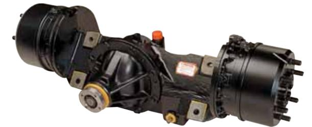
Splined side gear, drive hub gears transmit high torque to drive wheels
