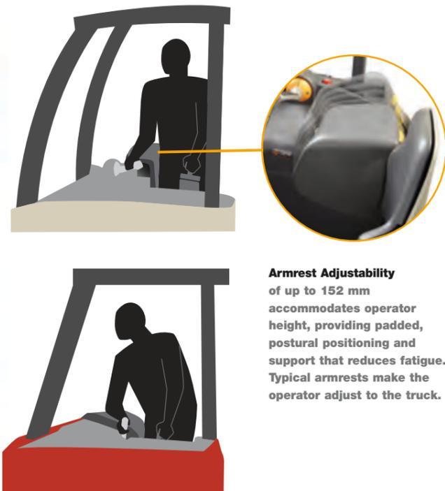
**Armrest Adjustability** of up to 152 mm accommodates operator height, providing padded, postural positioning and support that reduces fatigue. Typical armrests make the operator adjust to the truck.
