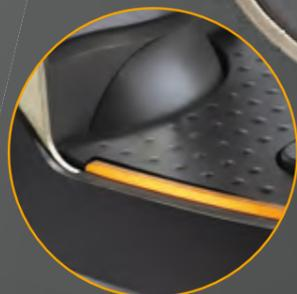
**Entry Bar® Safety Switch** – helps to improve operator safety by working in combination with the brake and presence pedal. If an operator places a foot on the entry bar switch, the lift truck automatically slows down and sounds an audible alarm.
