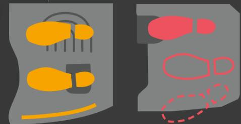
**Brake and Presence Pedal** – promotes safe operation with a dual-pedal design that discourages operators from using only one foot to operate the truck. Protects both the truck and the operator by automatically applying the brake when the operator's left foot is removed from the brake pedal. The roomier cabin and ability to adjust the position of the feet provide postural relief during travel.
