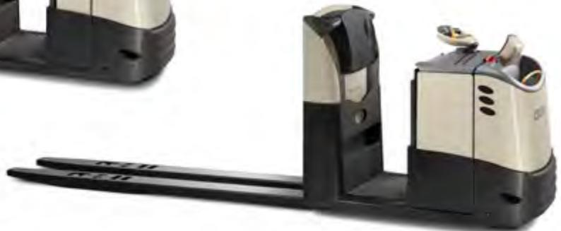
The GPC 3045 model elevates pallet loads weighing as much as 1200 kg up to 960 mm, providing ergonomic and productivity advantages.
