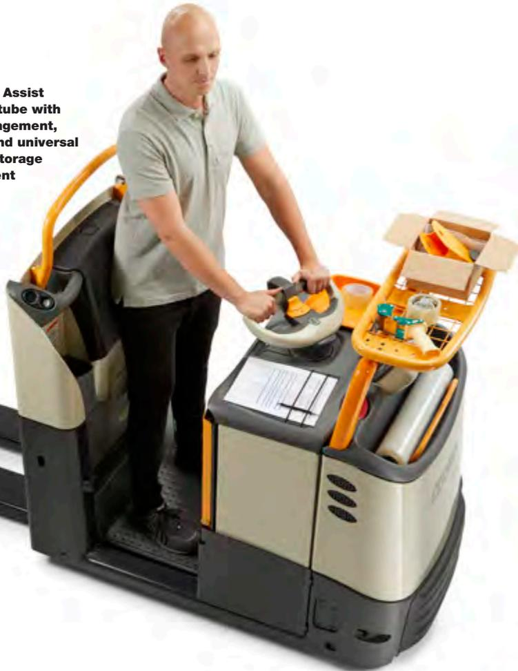
**A wide selection of Work Assist accessories adds to the exceptional performance and productivity advantages of the GPC 3000 Series. Crown engineers analysed the broad range of picking tasks and then designed Work Assist accessories which can be application-tailored to enhance convenience, comfort, safety and productivity.**
