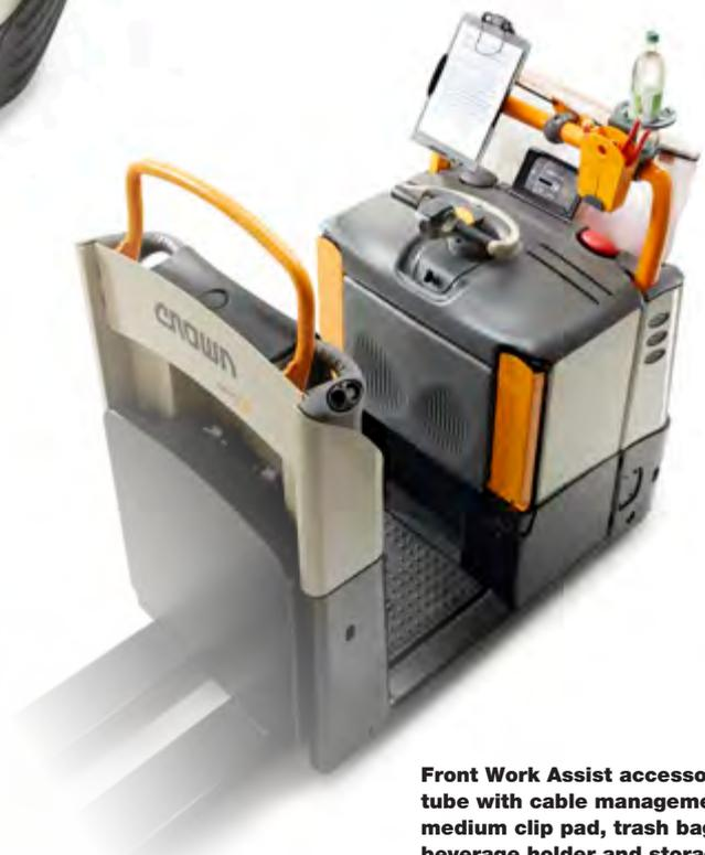
**Front Work Assist accessory tube with cable management, medium clip pad, trash bag and beverage holder and storage pouch**
