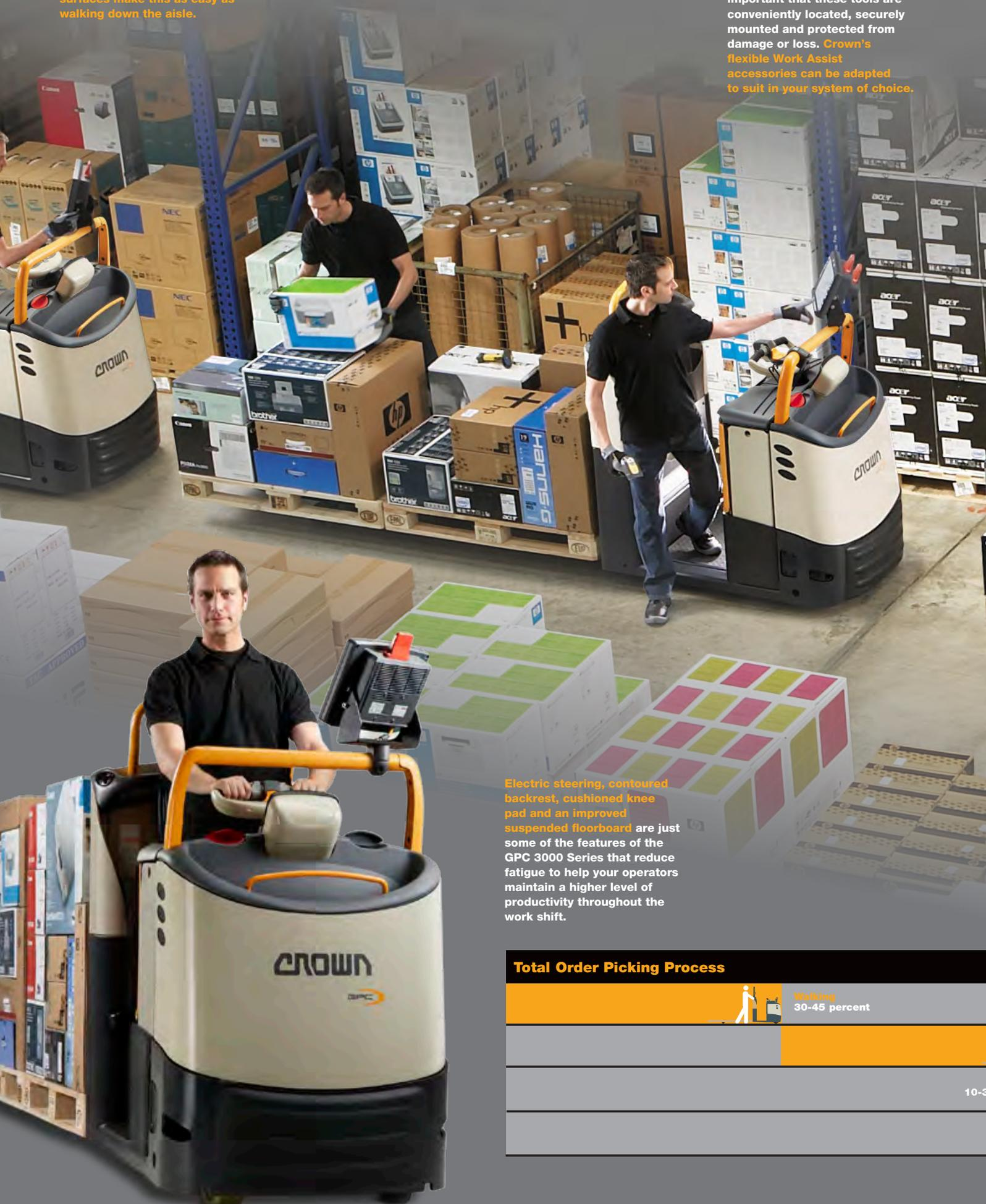
Electric steering, contoured backrest, cushioned knee pad and an improved suspended floorboard are just some of the features of the GPC 3000 Series that reduce fatigue to help your operators maintain a higher level of productivity throughout the work shift.
