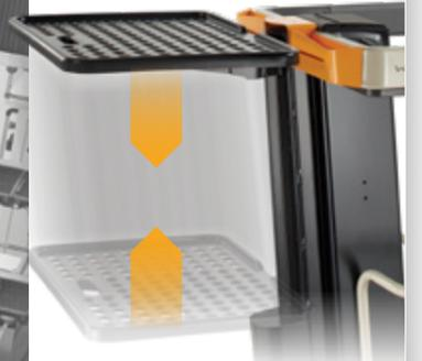
**Five-position manual load tray (standard)** accommodates loads of varying shapes and sizes. The tray can also be folded up and stowed away when higher loads are needed on the load deck.
