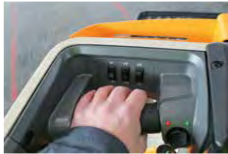
04 The left hand is used to steer, adjust the height of the load tray, engage "creep" mode and control the work lights
