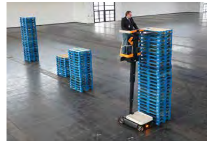
01 The operator platform can be raised hydraulically to a height of 2,995 mm
