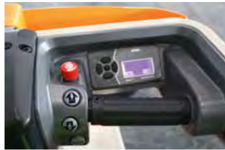
03 The travel speed and operator platform controls are positioned on the right-hand side of the cockpit
