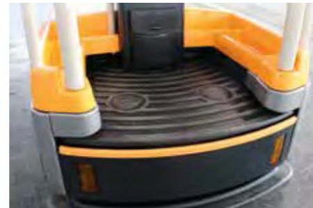
05 The operator platform provides secure footing – before the truck will start, the operator must deliberately step on the round markings
