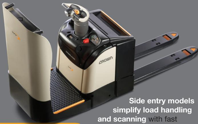
Side entry models simplify load handling and scanning with fast on/off access and shorter walking distance to pallets. The backrest offers added comfort, especially useful in order picking applications.
