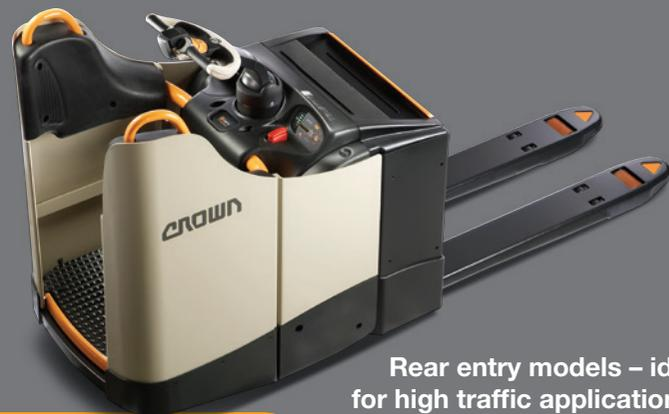
Rear entry models – ideal for high traffic applications and long run distances – provide operator comfort with extensive padding, built-in storage and rugged construction.
