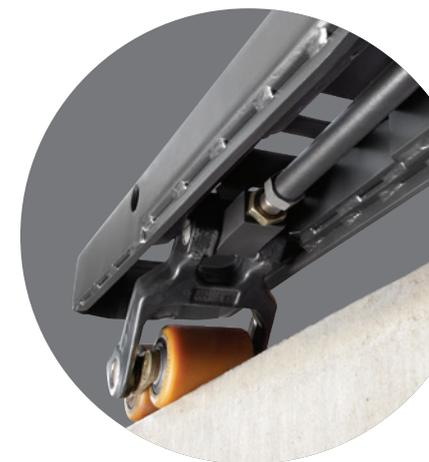
**One-piece high tensile steel forks** are formed into a C-channel and reinforced in critical areas. An adjustable pull-rod lift linkage eliminates buckling forces and elevates the riser axle for protection.
