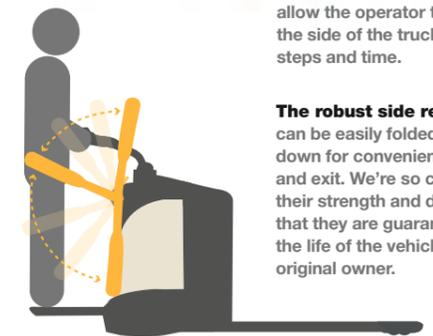
**The robust side restraints** can be easily folded up and down for convenient entry and exit. We're so confident in their strength and durability that they are guaranteed for the life of the vehicle for the original owner.
