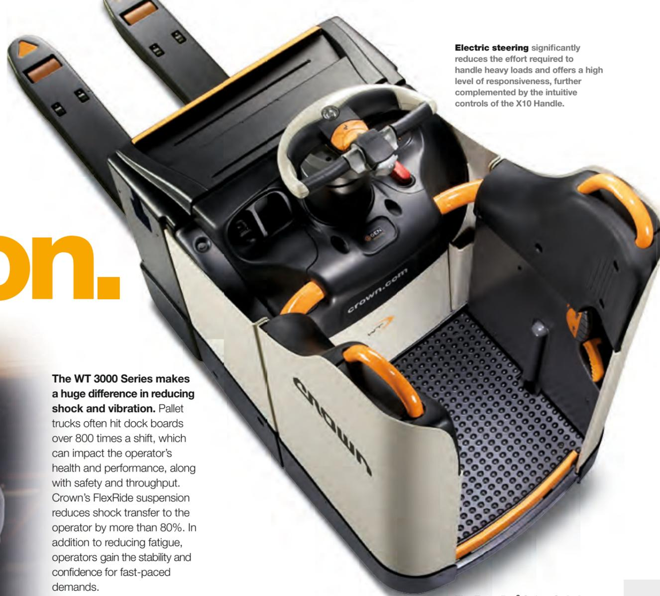
**Electric steering** significantly reduces the effort required to handle heavy loads and offers a high level of responsiveness, further complemented by the intuitive controls of the X10 Handle.
