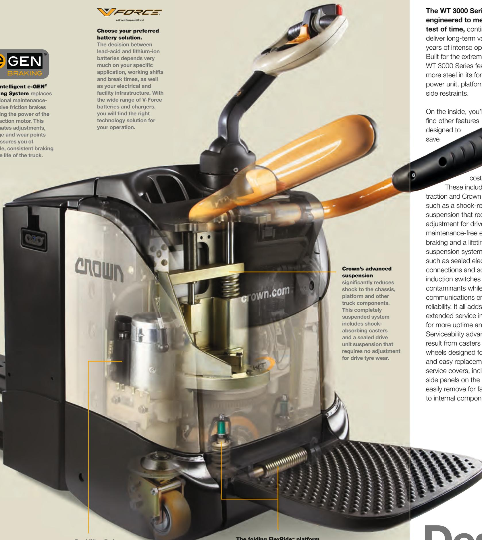
**Dual lift cylinders support each corner,** reducing stress and wear while also improving handling, especially on off-centre loads.
