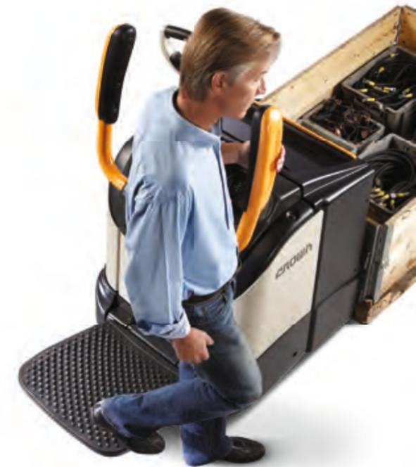
**Crown's side restraints** allow the operator to step off the side of the truck to save steps and time.
