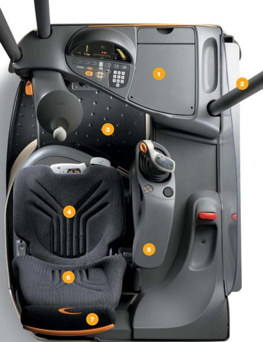
The MoveSeat swivels 10 degrees from the neutral position to enhance visibility when travelling power unit first. When travelling forks first, the seat swivels 20 degrees from the neutral position, enhancing forward and upward visibility to the forks.
