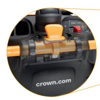
Heavy-duty side restraints feature 50 mm diameter heavy-wall steel tubing and rugged C-clamp mounting system.
