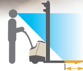
**The sloped, low-profile power unit and clear mast design** of the Crown Stacker Series provide excellent fork tip visibility (typically 50 percent of the total fork length).
