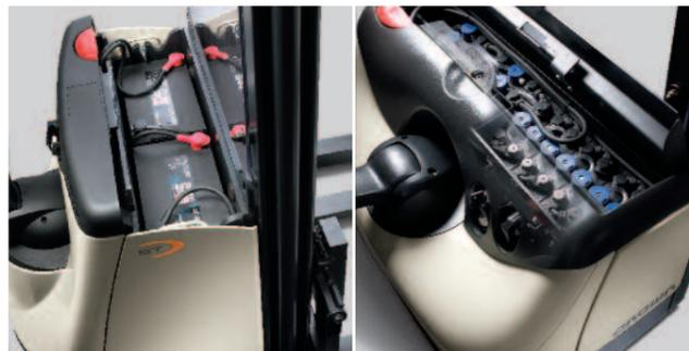
**Multiple battery options:** a variety of battery options are available including maintenance-free battery packs up to 192 Ah and industrial wet cell batteries up to 180 Ah (shown with optional central watering system).
