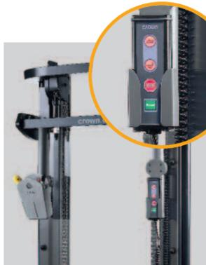
**Remote raise/lower control:** allows operator to control lift or lower function when using the stacker as a work positioner.
