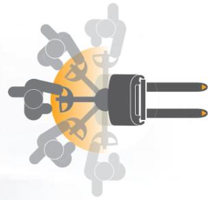
**The centre-mounted tiller on Crown stackers** positions the operator a safe distance from the power unit and provides better manoeuvrability and visibility.
