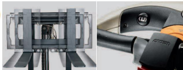
**Side shift with integrated control:** allows operator to shift the load left or right up to 100 mm. Side shift activation switch is integrated in Crown's X10 handle (SX only).
