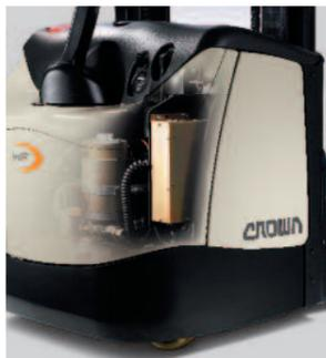
**Integrated battery charger:** solid-state 30 Amp high frequency battery charger is standard on all models.
