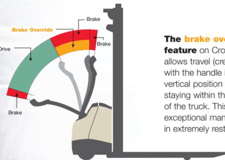
**The brake override feature** on Crown stackers allows travel (creep speed) with the handle in a near vertical position while staying within the geometry of the truck. This provides exceptional manoeuvrability in extremely restricted areas.
