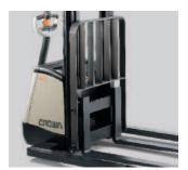
**Load backrest:** helps stabilise unsteady loads when travelling, lifting and lowering.
