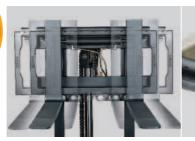
**Side shift with integrated control:** allows operator to shift the load left or right up to 100 mm. Side shift activation switch is integrated in Crown's X10 handle (SX only).
