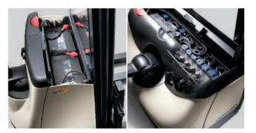
**Multiple battery options:** a variety of battery options are available including maintenance-free battery packs up to 190 Ah and industrial wet cell batteries up to 290 Ah (shown with optional central watering system).
