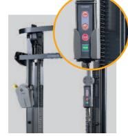
Remote raise/lower control\*: allows operator to control lift or lower function when using the stacker as a work positioner.
