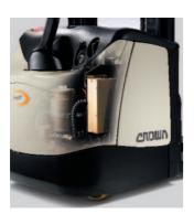
**Integrated battery charger:** solid-state 30 Amp high frequency battery charger.
