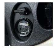
**Battery discharge indicator:** includes lift-lock-out and integrated hour metre.
