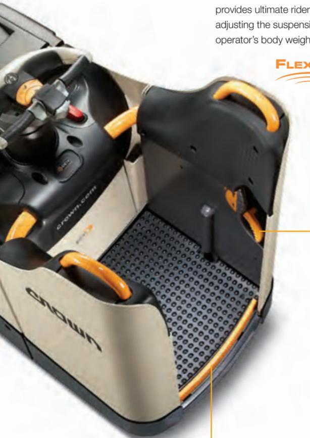
**The Entry Bar® Safety Switch** helps to promote operator safety. If an operator places a foot on the entry bar switch, the double stacker automatically slows down.
