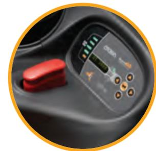
**Access 1 2 3 Comprehensive System Control** includes programmable performance settings to match the lift truck with operator skill levels or facility requirements.
