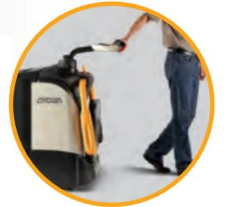
**Manoeuvrability** advantages result from the fold-up operator platform, contoured power unit and ergonomic tiller positioning providing ample foot clearance.
