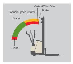
When entering the **Position Speed Control** zone, the travel speed in fork direction will be automatically reduced to 1.5 km/h without the need to come to a stop and a further command from the operator.
