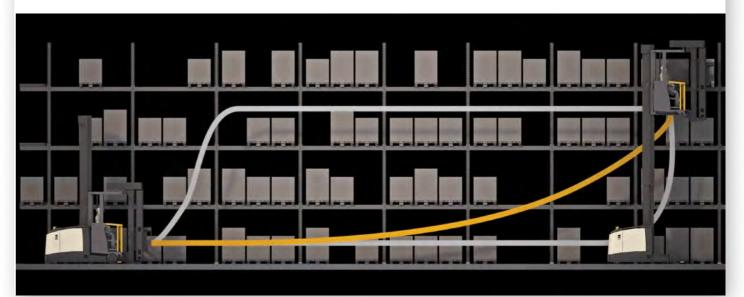
Auto Fence helps promote safety by slowing or stopping travel and limiting lift height within a very narrow aisle based on the lift truck's location.
