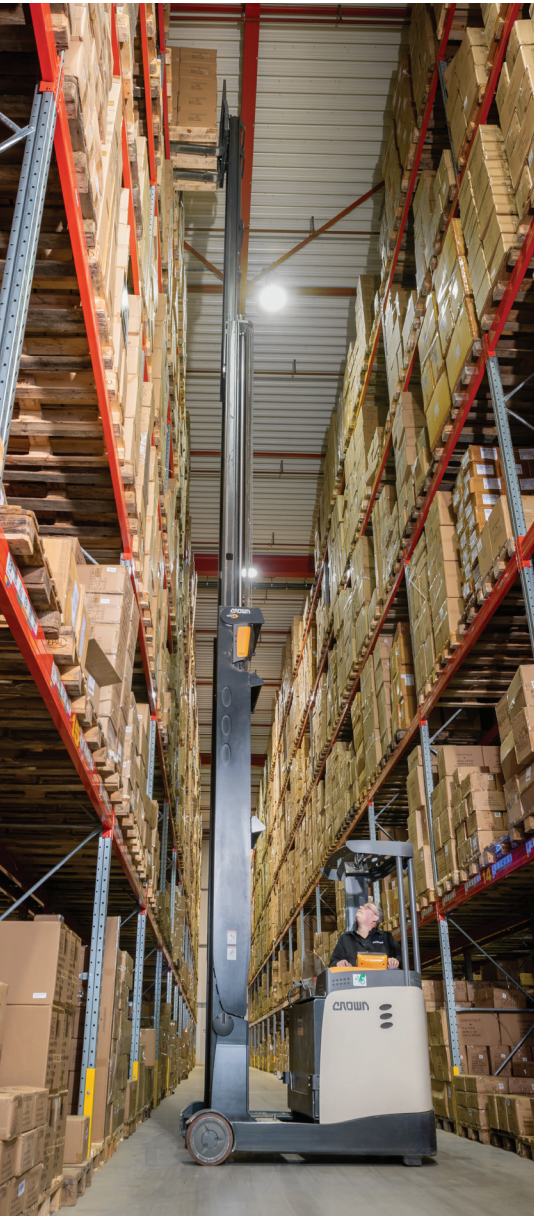
Xpress Lower technology doubles the lowering speed, thereby increasing productivity in the warehouse.
