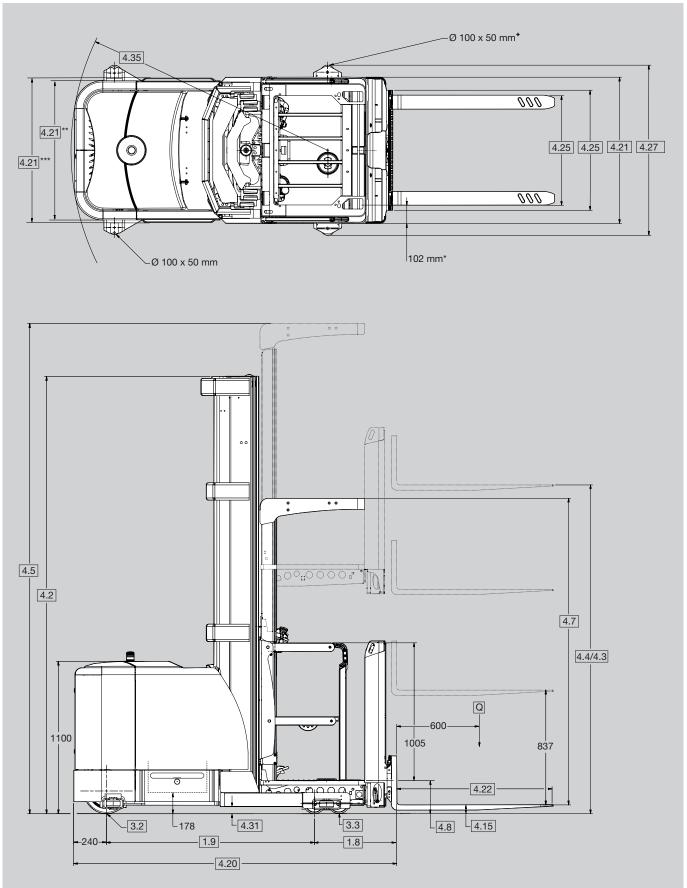
\* 140 mm when  $\underline{4.4}$  is greater than 6,910 up to 9,195 mm 203 mm when  $\underline{4.4}$  is greater than 9,195 mm \*\* Overall width front
