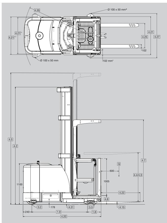
\* 140 mm when  $\boxed{4.4}$  is greater than 6,095 up to 8,840 mm 203 mm when  $\boxed{4.4}$  is greater than 8,840 mm
