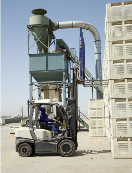
“Our forklifts experience quick runs in and out of the building in temperatures up to 110°F. This typically put a large strain on our forklift operations, but our C-5 trucks don't have a problem. With our previous forklifts, we had a lot of debris get stuck in the radiator and cause overheating. The C-5 solved this problem by reversing the fan every time the truck is started and this clears the debris.”
