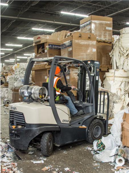
“The sealed brakes, the sealed undercarriage, and the fan system - the cooling system that the Crown’s have - have taken our maintenance costs way down. We’ve probably cut our cost over 50 to 60 percent.”
