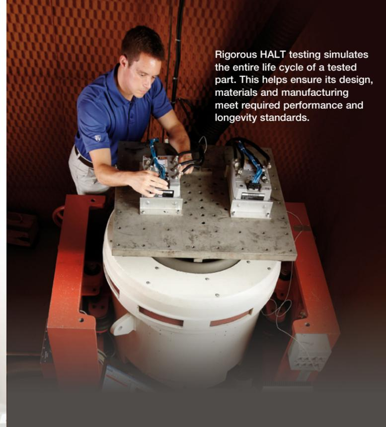
Electrical components on our lift trucks are tested at -40° to 85°C to verify longevity in extreme temperatures.
