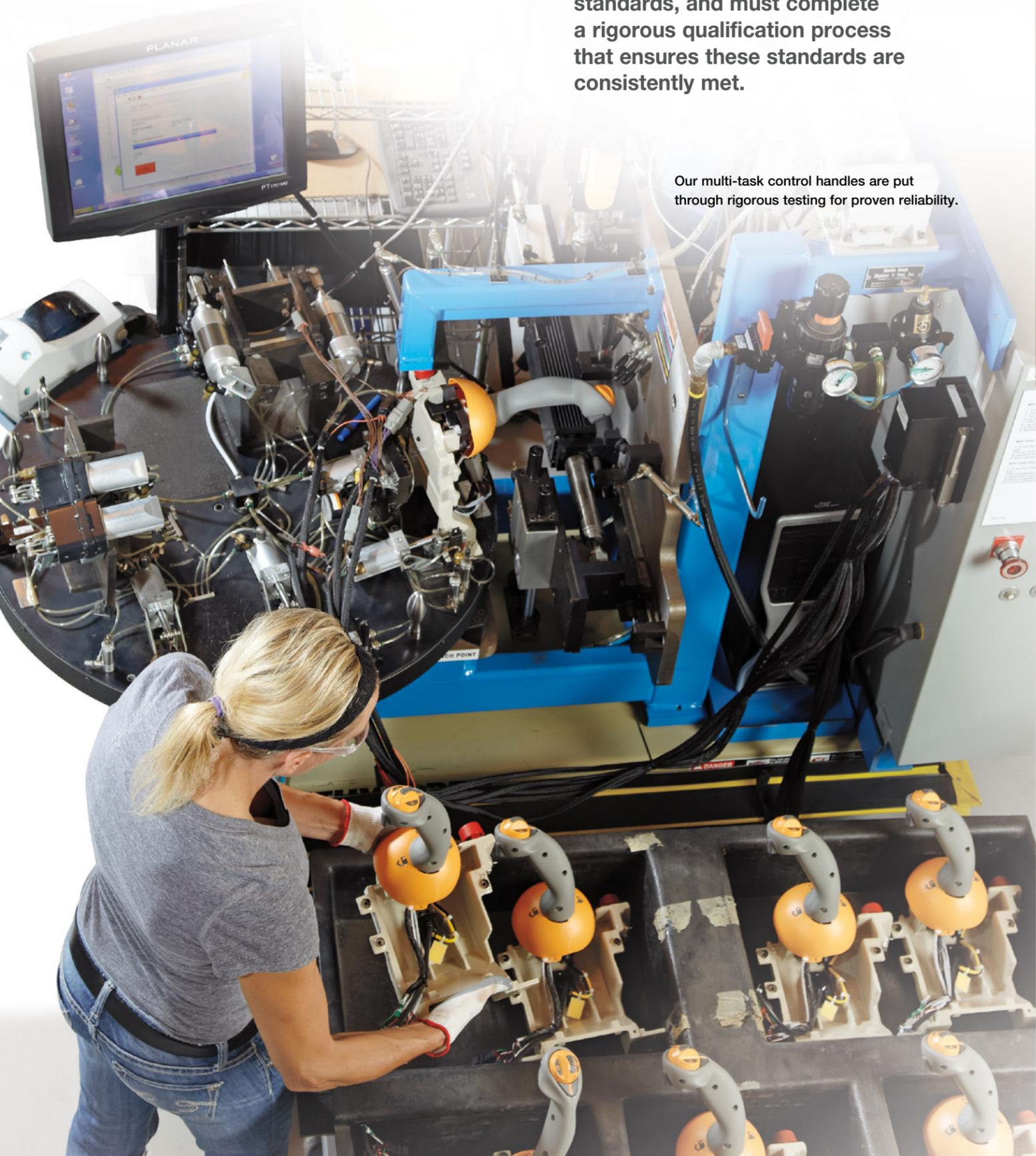
Rigorous HALT testing simulates the entire life cycle of a tested part. This helps ensure its design, materials and manufacturing meet required performance and longevity standards.
