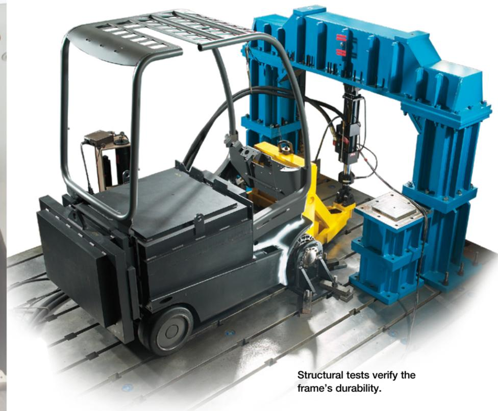
Structural tests verify the frame's durability.
