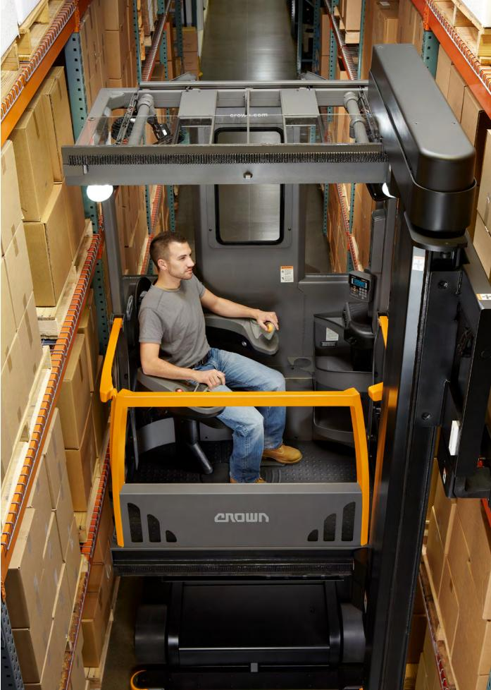
For example, the Crown RC Series of stand-up forklifts employ a contoured, low-profile power unit on the side where the operator is positioned to provide increased visibility during travel and a clear view of the forks when handling loads. Similarly, newer stockpickers feature expanded views through the platform window and on each side to facilitate order picking at height.
