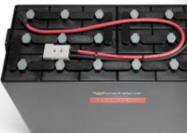
**Flat Plate** Traditional, time-tested design that employs heavy grid construction to limit corrosion and a five-layer wrap to minimize positive active material shedding. Cost-effective, yet still includes more active material for greater performance and capacity. Flat plate designs excel in high-charge return applications.
