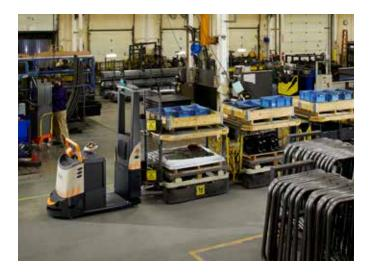
In select cases where the operations do not provide a clear path for the DualMode T tow tractor, the vehicle stops and notifies workers that action or attention is required. Since the vehicles feature dual modes of operation - automated and manual - any trained operator can manually move the vehicle and its cargo to its specified course and resume automated operation.
